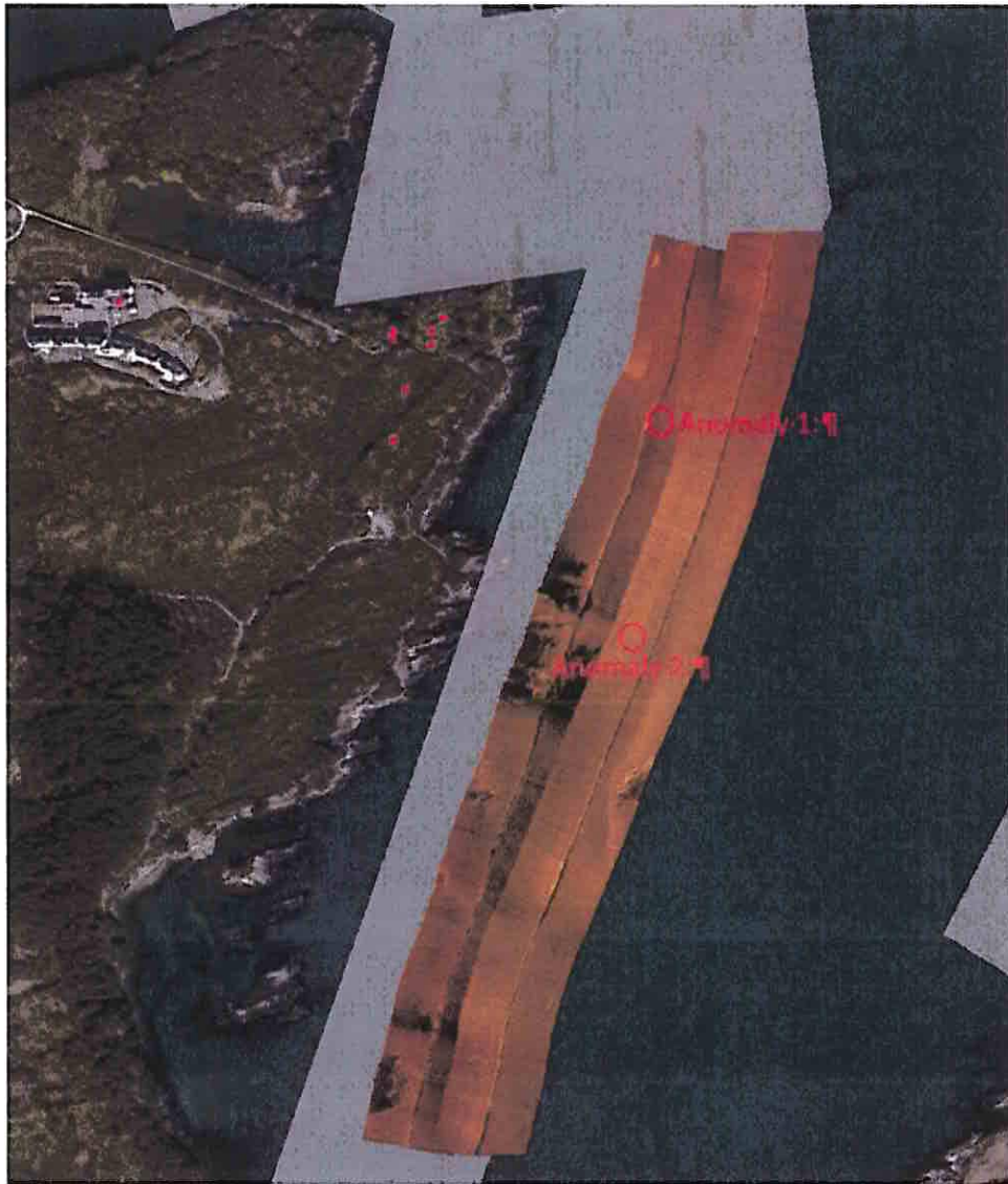
Figure 10: Side scan sonar image of T05/502 and T05/538 close to Dunboy, Berehaven.
